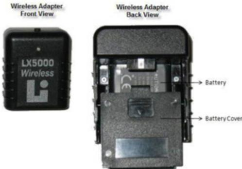
4. Slip the wireless adapter over the DAS module until it clicks into place.
