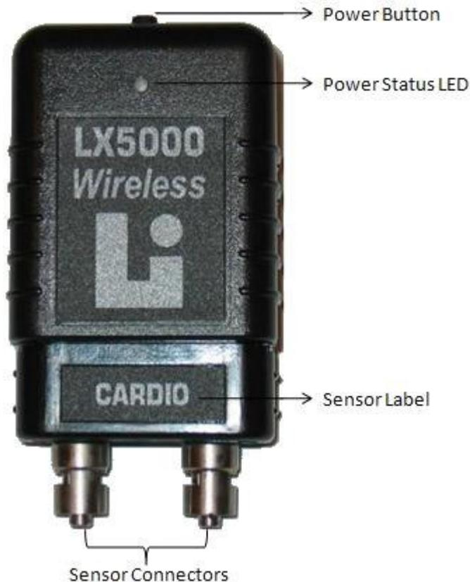
3. Turn the adapter on by pressing the power button until the power status LED flashes red then green. The adapter is now on and ready to use.
